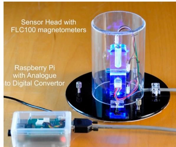
*Raspberry Pi computer attached to a three-axis magnetometer.*
