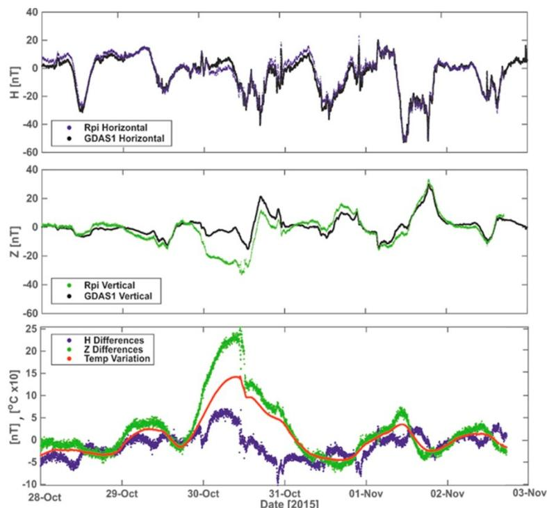
Variation in the Horizontal (upper panel) and Vertical (middle panel) components of the magnetic field for five days from 28th October to 2nd November 2015. Difference between GDAS1 and Raspberry Pi sensors in the H and Z component and the temperature variation (exaggerated  $\times 10$ ) are also shown (lower panel).
