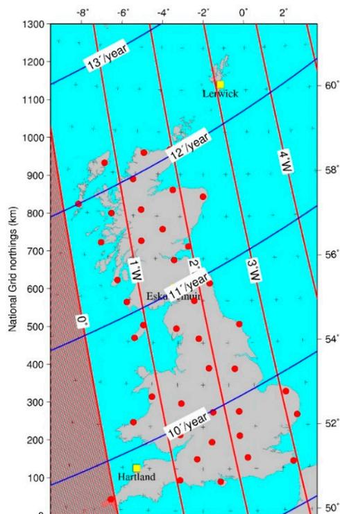
*Grid magnetic angle and its annual rate of change in 2015. The shaded area shows where magnetic north is east of grid north.*
