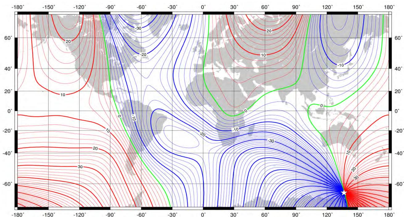
Declination (magnetic variation) at 2015.0 from the World Magnetic Model (WMM2015). Red - positive (east), blue - negative (west), green - zero (agonic line). Contour interval is  $2^\circ$ , white star is location of a magnetic pole and projection is Mercator. This is an example of an isogonic chart. Credit: British Geological Survey (Natural Environment Research Council).
