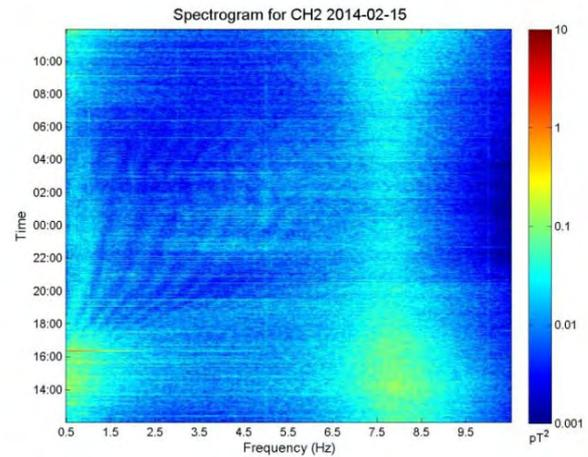
*Spectrogram for 15/16<sup>th</sup> March 2014. The wispy fringes between 18:00-04:00 and 1-5 Hz are the Ionospheric Alfvén Resonances. The first Schumann resonance is the diffuse region visible around 8 Hz*
